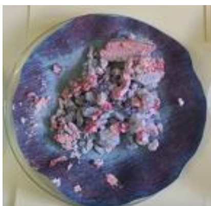
Figure 2. Synthesized complex of 2-acetoxy benzene carboxylic acid with Co (II) ion
