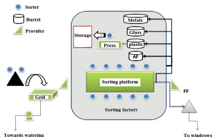
**Figure 8.** Sorting factory of the composting unit
