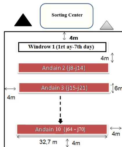
**Figure 9.** Arrangement of windrows in the fermentation area
